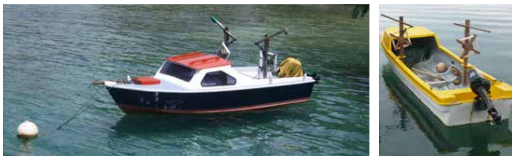
Figure 3: (a) 5-m Hartley model and (b) fiberglass boat. Both vessels are equipped with fishing reels and an outboard motor.
